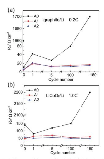
Fig. 2 EIS spectra of the graphite/Li and LiCoO2/Li half-cells with electrolytes AO, A1 and A2, after storage for 24 h, 1st, 5th, 100th and 160th cycles at 25 °C. Frequency range of 10<sup>-2</sup> Hz to 10<sup>5</sup> Hz with a potential amplitude of 5 mV. (a) The change of the charge-transfer resistances ( $R_{ct}$ ) in the graphite/Li cells. (b) The change of  $R_{ct}$  in the LiCoO2/Li cells.
