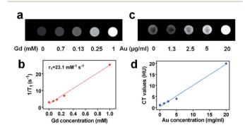
Fig. 2 (a)  $T_1$ -Weighted MR images of TGP-PEG-Gd solutions. (b) Linear fitting of  $1/T_1$  values as a function of the Gd concentration. (c) CT images of TGP-PEG-Gd solutions. (d) Linear fitting of CT values (HU) as a function of the Au concentration.
