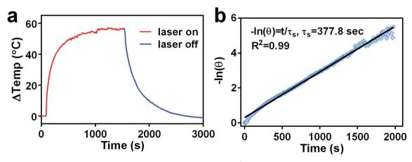
Fig. 4 (a) Heating (irradiated with a 660 nm laser at a power density of 1.0 W cm<sup>-2</sup>) and cooling (without laser irradiation) curves of a solution of TGP-PEG-Gd with an Au concentration of 5  $\mu$ g mL<sup>-1</sup>. (b) Linear fit of the negative natural logarithm of the driving force temperature as a function of time.
