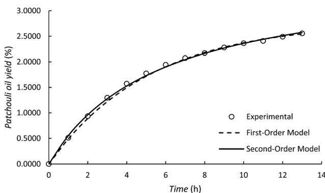
**Fig. 8** A comparison of the first-order and second-order kinetic models with the experimental results for the extraction of patchouli oil by the conventional method (hydrodistillation). The ratio of patchouli leaves to distilled water was 0.10 g mL<sup>-1</sup>.
