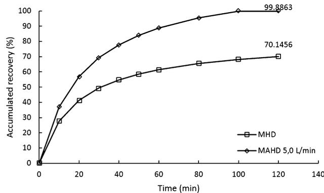
Fig. 5 Accumulated recovery of patchouli oil obtained by microwave hydrodistillation (MHD) and microwave air-hydrodistillation (MAHD; air flow rate 5.0 L min<sup>-1</sup>). The microwave power was 600 W and the ratio of patchouli leaves to distilled water was 0.10 g mL<sup>-1</sup>.
