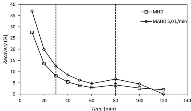
Fig. 6 Recovery of patchouli oil obtained by microwave hydrodistillation (MHD) and microwave air-hydrodistillation (MAHD; air flow rate 5.0 L min<sup>-1</sup>). The microwave power was 600 W and the ratio of patchouli leaves to distilled water was 0.10 g mL<sup>-1</sup>.
