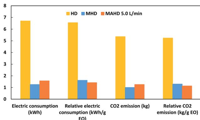
Fig. 9 The electric consumption and environmental impact (CO<sub>2</sub> emissions) for the extraction of patchouli oil by the conventional method (hydrodistillation; HD), the microwave hydrodistillation method (MHD) and the microwave air-hydrodistillation method (MAHD; air flow rate 5.0 L min<sup>-1</sup>). The microwave power was 600 W and the ratio of patchouli leaves to distilled water was 0.10 g mL<sup>-1</sup>.
