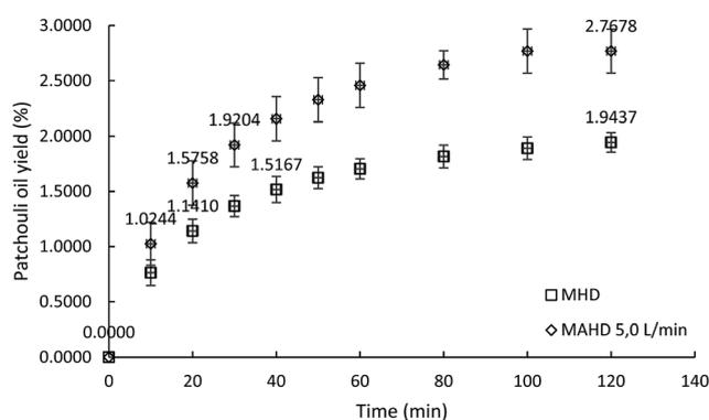
Fig. 4 Comparison between the yields of patchouli oil obtained by microwave hydrodistillation and microwave air-hydrodistillation (air flow rate 5.0 L min<sup>-1</sup>). The microwave power was 600 W and the ratio of patchouli leaves to distilled water was 0.10 g mL<sup>-1</sup>.
