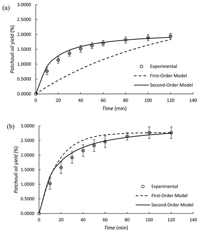
**Fig. 7** A comparison of the first-order and second-order kinetic models with the experimental results for the extraction of patchouli oil by (a) microwave hydrodistillation and (b) microwave air-hydro-distillation (air flow rate 5.0 L min<sup>-1</sup>). The microwave power was 600 W and the ratio of patchouli leaves to distilled water was 0.10 g mL<sup>-1</sup>.
