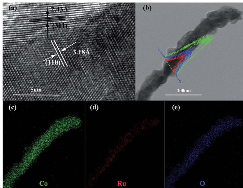
Fig. 4 HRTEM of S-6 (a); TEM image of the RuO<sub>2</sub>/Co<sub>3</sub>O<sub>4</sub> nanocrystalline-scan EDS analysis across the nanocrystal (b); elemental mappings of Co (c); Ru (d); O (e).
