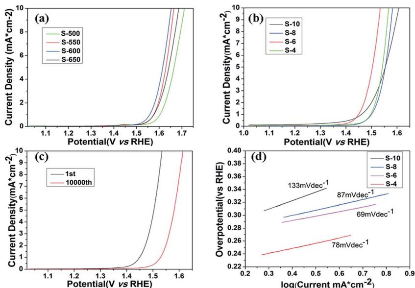
Fig. 5 OER polarization curves of Co<sub>3</sub>O<sub>4</sub> samples annealed at different temperature (a); and RuO<sub>2</sub>/Co<sub>3</sub>O<sub>4</sub> complex with different molar ratios (b) in 1 M KOH; polarization curves of S-6 after the 1st and 10 000th cycles (c); Tafel plots of S-4, S-6, S-8, and S-10 (d).
