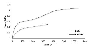
Fig. 6 Mechanical properties of PAA and PAA-HB hydrogels.
