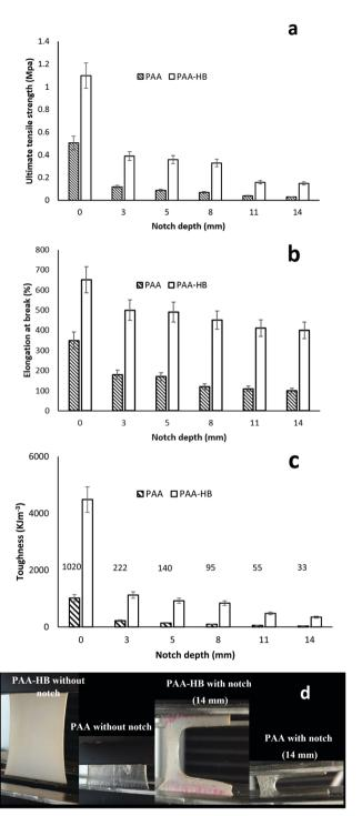
Fig. 8 Comparison of the mechanical properties of PAA with PAA-HB hydrogel for different notch depths. (a) Ultimate tensile strength, (b) elongation at break and (c) toughness. Figure (d) shows the stretchability of the intact sample (un-notched) *versus* the notched sample (14 mm) for both PAA and PAA-HB hydrogels.
