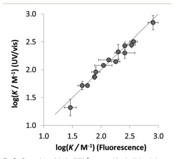
Fig. 3 Comparison of the  $\log(K/M^{-1})$  measured for the H-bonded complexes  $1\cdot X$  using fluorescence emission spectroscopy and UV/vis absorption spectroscopy. The line represents  $\log(K/M^{-1})$  (fluorescence) =  $\log(K/M^{-1})$  (UV/vis).
