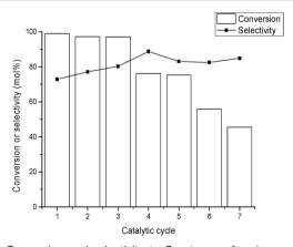
Fig. 4 Conversion and selectivity to 3-octanone for six consecutive catalytic runs. The reaction was carried out at 120  $^{\circ}$ C under an inert atmosphere (N<sub>2</sub>, 2 bar) using isopropanol as solvent.
