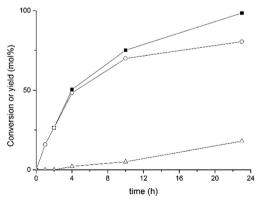
Fig. 3 Conversion of 1-octen-3-ol over Ir@CTF (squares) and evolution of products: 3-octanone (circles) and 3-octanol (triangles). The reaction was carried out at 120  $^{\circ}$ C under an inert atmosphere (N<sub>2</sub>, 2 bar) using isopropanol as solvent.
