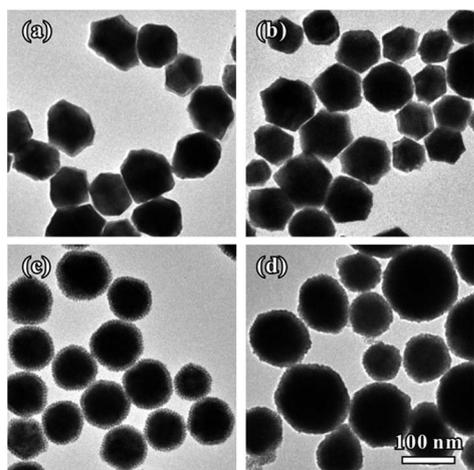
Fig. 4 TEM images of the Au–Pt bimetallic NCs that were prepared using the standard procedure, except for variation in the introduced amount of  $\text{K}_2\text{PtCl}_4$  (1 mM): (a) 0.5 mL, (b) 1.0 mL, (c) 2.0 mL and (d) 3.0 mL.
