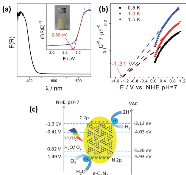
Fig. 1 (a) UV-vis DRS spectrum of  $g\text{-C}_3\text{N}_4$  polymers; inset: the corresponding Tauc plot. (b) Mott–Schottky plots of the  $g\text{-C}_3\text{N}_4$  electrode in 0.2 M  $\text{Na}_2\text{SO}_4$ , pH = 7. (c) Band structure diagram of  $g\text{-C}_3\text{N}_4$  polymers calculated by optical absorption and typical electrochemical Mott–Schottky methods.
