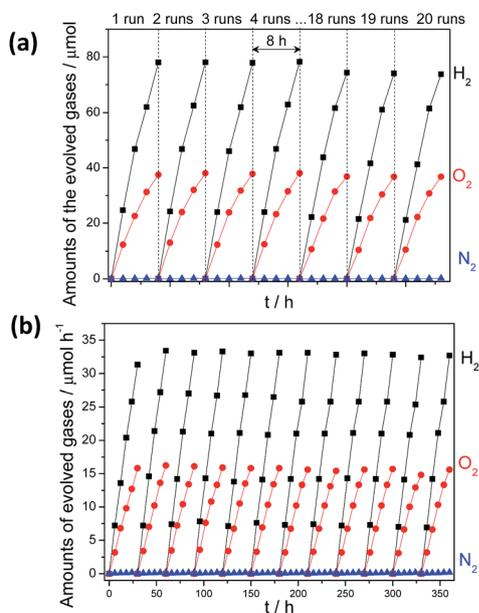
Fig. 4 Time course of water splitting activities of 3 wt% Pt,  $\text{PtO}_x$  and 1 wt%  $\text{CoO}_x$  Co-modified  $\text{g-C}_3\text{N}_4$  polymers under (a) UV-vis ( $\lambda > 300$  nm) irradiation and (b) visible light ( $\lambda > 420$  nm) irradiation.
