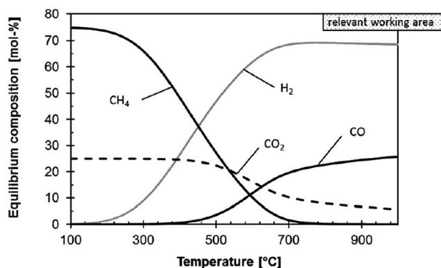
Fig. 2 Influence of temperature on the thermodynamic equilibrium of the rWGS reaction at 1 bar and H<sub>2</sub>/CO<sub>2</sub> molar ratio of 3/1. Reproduced with permission from John Wiley and Sons (from ref. 17).
