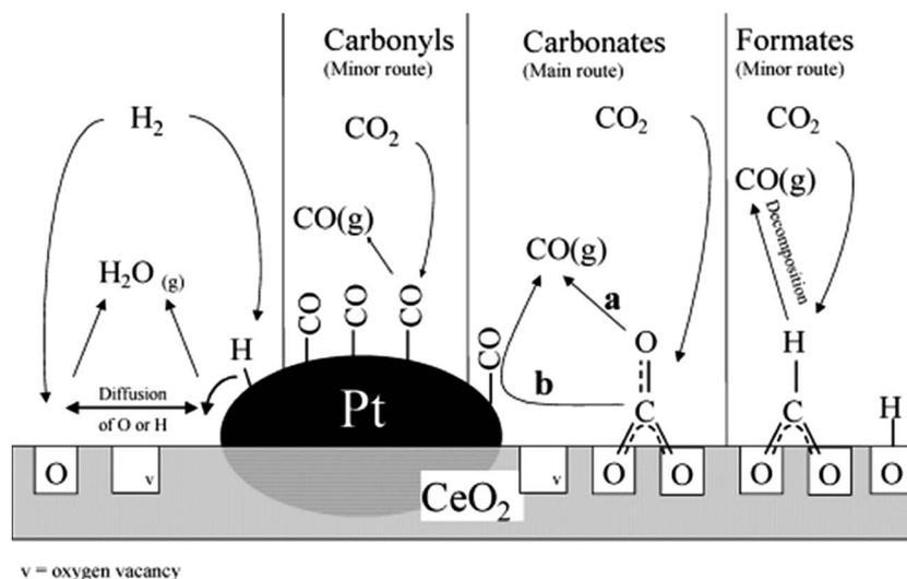
Fig. 7 Proposed rWGS mechanism on the Pt/CeO<sub>2</sub> interface. Reproduced with permission from the American Chemical Society (from ref. 109).
