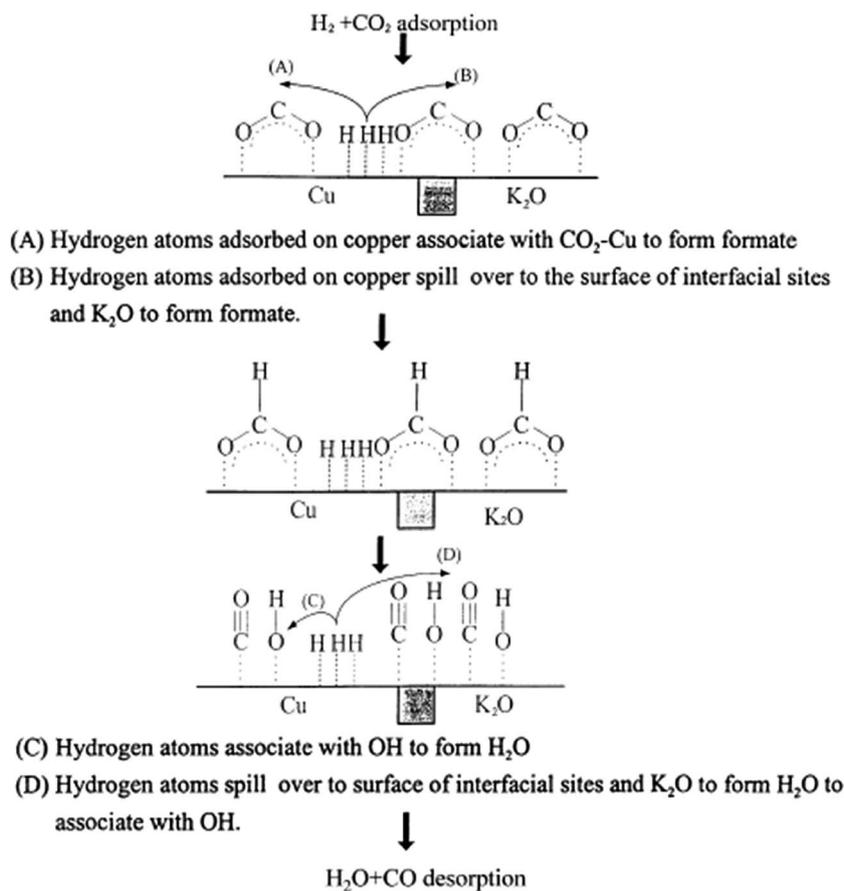
Fig. 6 Proposed rWGS mechanism on the Cu/K/SiO<sub>2</sub> interface. Reproduced with permission from Elsevier (from ref. 99).
