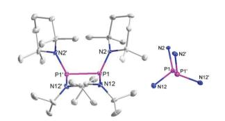
Fig. 2 Representation of the molecular structure of {9}2 in the crystal (left) and reduced plot of the central P2N4 skeleton (right). Thermal ellipsoids were drawn at 50% probability level, and H atoms were omitted for clarity. Selected bond lengths [Å]: P1-N12 1.727(5), P1-N2 1.738(5), P1-P1' 2.357(2), P1'-N12' 1.711(5), P1'-N2' 1.740(5).
