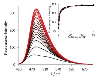
Fig. 4 Fluorescence emission spectra of 1.Zn<sub>2</sub> (5 μM) in response to PPI  $(0-300 \mu M)$  in HEPES (5 mM, 145 mM NaCl, pH 7.4) at 25 °C.  $\lambda_{ex}$  = 390 nm, slits = 5 nm/5 nm. Inset: Binding isotherm (-) obtained by fitting the observed fluorescence intensities at 480 nm (●) to a 1:1 binding model using non-linear regression
