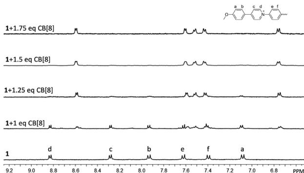
**Fig. 1** Partial  $^1\text{H}$  NMR spectra of **1** and CB[8] at different molar ratios in  $\text{D}_2\text{O}-\text{CD}_3\text{OD}$  (17 : 3, V/V) at 25 °C. The concentration of **1** was fixed at 1.0 mM.
