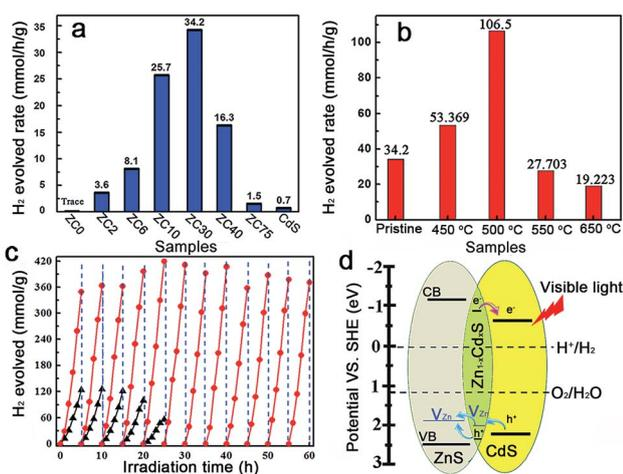
Fig. 3 (a) Photocatalytic H<sub>2</sub>-production activities of the ZCX samples and (b) ZC30 post-annealed at different temperatures in a 0.35 M Na<sub>2</sub>S and 0.25 M Na<sub>2</sub>SO<sub>3</sub> mixed aqueous solution under visible-light irradiation. (c) Comparison of the photocatalytic stabilities of pristine ZC30 (triangle) and ZC30-500 (circle). (d) Schematic illustrating charge transfer and separation in ZnS/Zn<sub>1-x</sub>Cd<sub>x</sub>S/CdS.
