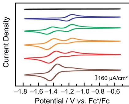
Fig. 3 Cyclic voltammograms under Ar at  $100 \text{ mV s}^{-1}$  in DMF, TBAPF<sub>6</sub> 0.1 M, on a glassy carbon electrode of a solution of 2 mM tpy (— black) and 2 mM tpy with added 1 mM (— blue), 2 mM (— green), 3 mM (— orange), 4 mM (— red) and 10 mM (— brown) of CoCl<sub>2</sub>.
