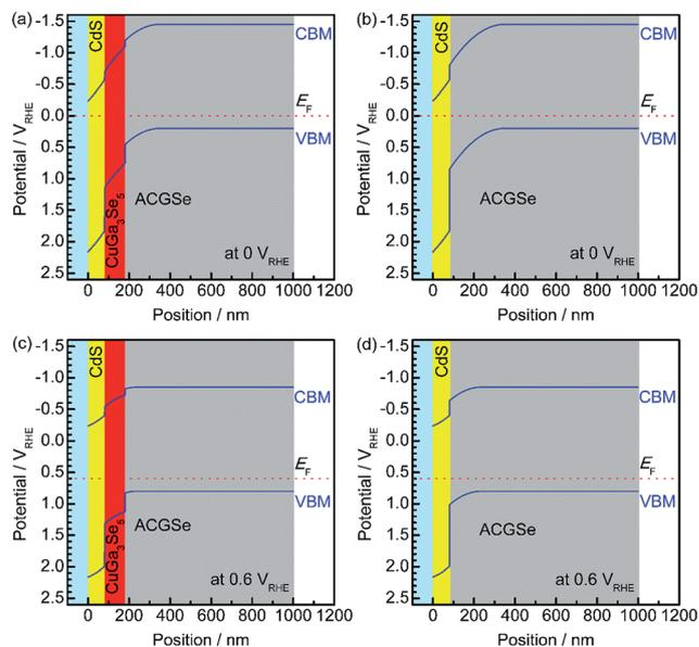
Fig. 8 Calculated band alignment near the solid–liquid interface for CdS/CuGa<sub>3</sub>Se<sub>5</sub>/ACGSe with CuGa<sub>3</sub>Se<sub>5</sub> deposited for 15 min, and Pt/CdS/ACGSe at an applied potential of 0 V<sub>RHE</sub> (a) and (b), and 0.6 V<sub>RHE</sub> (c) and (d). VBM, CBM and E<sub>F</sub> denote the valence-band maximum, conduction-band minimum, and Fermi energy, respectively.
