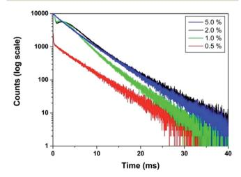
Fig. 10 PL decay curves of LaPO<sub>4</sub>:Eu $^{3+}$  samples (Eu $^{3+}$  mol% = 0.5, 1.0, 2.0, 5.0) (monitored at 592 nm and excited at 256 nm).
