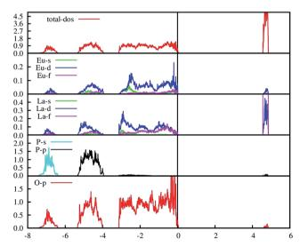
Fig. 13 PAW-PBE calculated total and angular momentum decomposed DOS of Eu<sup>3+</sup>-doped LaPO<sub>4</sub> (doping level is 6.25% at La<sup>3+</sup> position).
