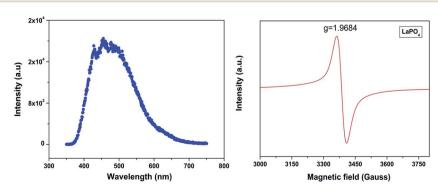
Fig. 4 (a) Emission spectrum of undoped LaPO<sub>4</sub> nanoparticles ( $\lambda_{\rm ex}$  – 230 nm) and (b) room-temperature EPR spectra of undoped LaPO<sub>4</sub>.
