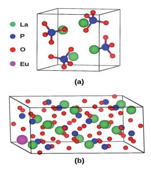
Fig. 11 (a) Unit cell of LaPO<sub>4</sub> (24 atoms) and (b) Eu<sup>3+</sup>-doped  $2 \times 2 \times 1$ supercell (96 atoms) of LaPO<sub>4</sub>.
