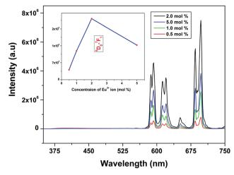
Fig. 9 PL emission spectra (corrected w.r.t. source) of LaPO<sub>4</sub>:Eu<sup>3+</sup> phosphors (mol% of Eu<sup>3+</sup> = 0.5, 1.0, 2.0, 5.0) excited at 256 nm. The insets show the PL emission intensities of  $^5D_0-^7F_1$  as a function of Eu<sup>3+</sup> ion concentration.
