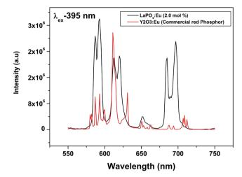
Fig. 18 Comparison of emission spectra of commercial red phosphor (Y<sub>2</sub>O<sub>3</sub>:Eu from Nichia Corporation, Japan) and LaPO<sub>4</sub>:Eu<sup>3+</sup> (2.0 mol%) under 395 nm excitation. The comparison is made on corrected spectra and integral intensity of all the peak is considered.
