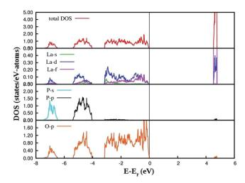
Fig. 12 PAW-PBE calculated total and angular momentum decomposed DOS of LaPO<sub>4</sub>.
