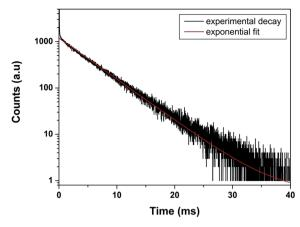
Fig. 8 Photoluminescence decay profile of LaPO<sub>4</sub>:Eu<sup>3+</sup> (0.5 mol%) at emission and excitation wavelength of 593 and 256 nm, respectively.
