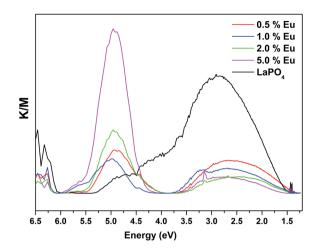
Fig. 15 UV-Vis absorption-energy curves of LaPO<sub>4</sub> and La<sub>1-x</sub>Eu<sub>x</sub>PO<sub>4</sub>.
