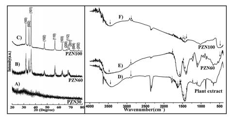
Fig. 2 (A), (B) and (C) XRD of PZN30, PZN60 and PZN100 respectively showing appearance of peaks for ZnO at higher temperature; (D), (E) and (F) FTIR spectra of lyophilized plant extract, PZN60 and PZN100 respectively showing appearance of transmittance bands (with arrow) for different functional groups of plant extract associated with ZnO NPs.
