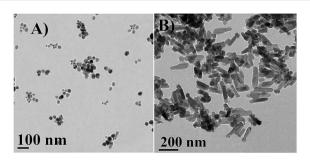
Fig. 4 HRTEM micrograph of synthesized ZnO. (A) Isolated spherical particles of PZN60, size ranging from 12-46 nm at 100 nm scale bar; (B) dumbbell shaped particles of PZN100, size ranging from 190-250 nm in lengths and 50-60 nm in breadths at 200 nm scale bar.
