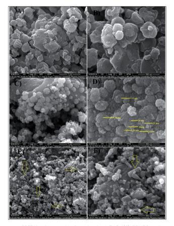
Fig. 3 FESEM micrograph of synthesized ZnO. (A) PZN30 at 1  $\mu$ m scale; (B) PZN30 at 500 nm scale; for PZN60 particles were spherical in nature and each particle was aggregation of many smaller particles. (C) PZN60 at 1  $\mu$ m scale; (D) PZN60 at 500 nm scale. For PZN100 dumbbell shaped larger particles due to crystal growth. (E) PZN100 at 1  $\mu$ m scale; (F) PZN100 at 500 nm scale.
