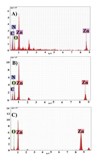
Fig. 5 EDX spectra of sample (A) PZN30, (B) PZN60 and (C) PZN100.
