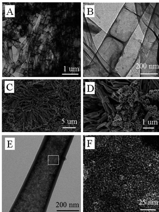
**Fig. 5** TEM (A and B) and SEM (C and D) images of micro/mesoporous nitrogen doped carbon nanotubes prepared by carbonization of PCMVImTf<sub>2</sub>N at 800 °C by using AAO as a template. (E and F) TEM images of micro/mesoporous nitrogen doped carbon nanotubes loaded with Fe<sub>2</sub>O<sub>3</sub> nanoparticles.
