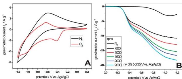
**Fig. 6** (A) Comparison of cyclic voltammograms of CNT@Fe<sub>2</sub>O<sub>3</sub> composites at 100 mV s<sup>-1</sup> after 20 min purge with N<sub>2</sub> (black) and O<sub>2</sub> (red) in 0.1 M KOH. (B) Linear sweep voltammograms at different rotational speeds recorded at 10 mV s<sup>-1</sup> in oxygen saturated 0.1 M KOH.
