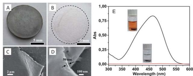
**Fig. 7** (A and B) Photographs of a carbonized thin film (ca. 50 nm thick) on a KBr disk and floating on water. (C and D) SEM images of the as-synthesized carbon thin films. (E) UV-Vis absorption and optical photographs of methyl orange aqueous solution (0.01 mg ml<sup>-1</sup>) before (black) and after (red) being treated with a micro/mesoporous nitrogen doped carbon film (100 μm thick).
