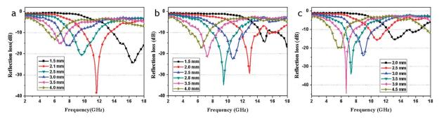
Fig. 10 The calculated reflection losses for RGO-Fe<sub>3</sub>O<sub>4</sub>-1 (a), RGO-Fe<sub>3</sub>O<sub>4</sub>-2 (b) and RGO-Fe<sub>3</sub>O<sub>4</sub>-3 (c) with different thicknesses in the frequency range of 2–18 GHz.
