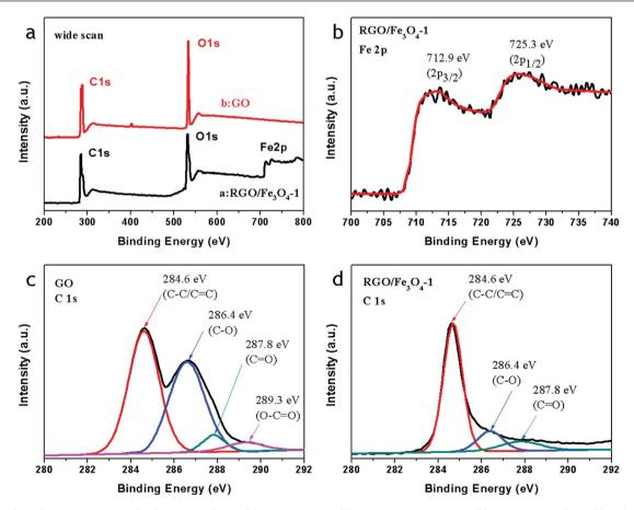
Fig. 3 X-ray photoelectron spectroscopy (XPS) spectra: wide scan (a), Fe 2p spectrum of the RGO– $Fe_3O_4$ -1 composite (b), C 1s spectrum of RGO (c), and C 1s spectrum of the RGO– $Fe_3O_4$ -1 composite (d).
