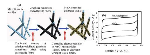
Fig. 9 (a) Schematic illustration of two key steps for preparing hybrid  $MnO_2$ -nanostructured textiles@graphene and (b) CV curves of an optimized  $MnO_2$ @graphene at different potential windows at the scan rate of 20 mV s<sup>-1</sup> in 1 mol l<sup>-1</sup>  $Na_2SO_4$  solution (modified from ref. 8a and 8b, respectively).
