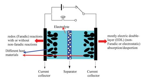
Fig. 1 Schematic illustration of ASCs.
