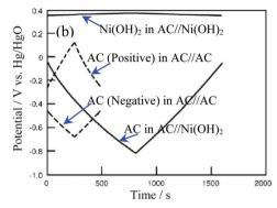
Fig. 15 (a) CV curve of Ni(OH)<sub>2</sub> in alkaline solution and (b) charge/discharge curves of the positive and negative electrodes in the AC//Ni(OH)<sub>2</sub> ASC and electric double layer capacitors of AC//AC at 1 mA cm<sup>-2</sup> in 10 mol l<sup>-1</sup> KOH aqueous solution (modified from ref. 87b and 90c).
