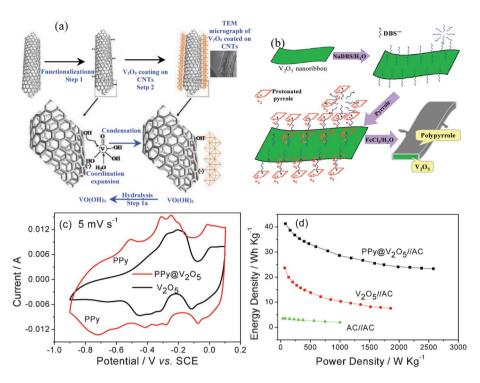
Fig. 3 Schematic illustration for the synthesis of (a)  $V_2O_5$ @CNTs (modified from ref. 37a) and (b)  $PPy@V_2O_5$ , (c) CV curves of  $V_2O_5$  and  $PPy@V_2O_5$  in 0.5 mol  $I^{-1}$   $K_2SO_4$ solution, and (d) Ragone plots of the ASC of  $V_2O_5$ //AC and  $PPy@V_2O_5$ //AC using 0.5 mol  $I^{-1}$   $K_2SO_4$  solution as the electrolyte (The capacitance and energy densities were calculated based on the total mass of two active electrode materials) (modified from ref. 6b).
