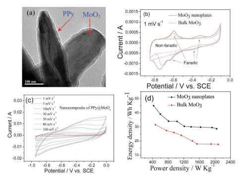
Fig. 4 (a) TEM micrograph of PPy coated MoO<sub>3</sub> nanorods, (b) CV curves of the bulk and nanoplates MoO<sub>3</sub>, (c) CV curves of the PPy@MoO<sub>3</sub> nanocomposite at different scan rate and (d) Ragonne plot of the ASCs based on MoO<sub>3</sub>//AC in 0.5 mol I<sup>-1</sup> Li<sub>2</sub>SO<sub>4</sub> solution (modified from ref. 6c and 49c).
