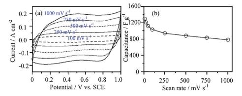
Fig. 8 (a) CV curves at different scan rates and (b) dependence of the capacitance on the scan rate for an annealed  $RuO_2 \cdot xH_2O$  nanotube arrayed electrode (0.19 mg cm<sup>-2</sup>) in 1.0 mol l<sup>-1</sup> H<sub>2</sub>SO<sub>4</sub> solution (modified from ref. 54a).
