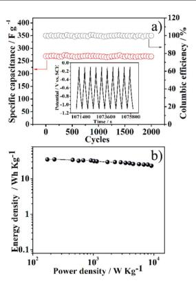
**Fig. 6** a) Variations of specific capacitance and the coulombic efficiency *versus* the cycle number of NGS-1 measured at a current density of  $1 \text{ A g}^{-1}$  within the potential range from -1.1 to -0.1 V. The inset shows the charge–discharge curves of the last 10 cycles for NGS-1. b) Ragone plots of supercapacitors composed of NGS-1 as positive and negative electrodes in 6 M KOH electrolyte.
