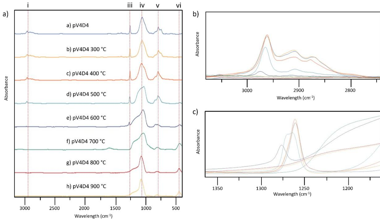
**Figure 3:** a) Ex-situ IR absorbance spectra showing the transformation of the PECVD-deposited pV4D4 polymer during pyrolysis; b) expanded view of the IR region from 2750 to 3100 cm<sup>-1</sup> showing the polyethylene stretching band; c) expanded view of the IR region from 1200 to 1300 cm<sup>-1</sup> showing the methyl stretching band.
