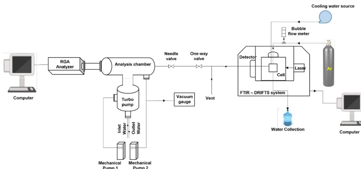
**Figure 1:** Schematic of the combined DRIFTS-RGA apparatus
