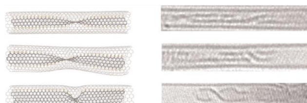
Fig. 10 TEM images of GNRs with different widths inside nanotubes. Reprinted with permission from ref. 134. Copyright 2012 American Chemical Society.
