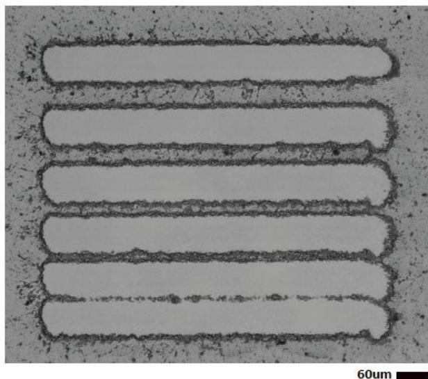
**Fig. 2** Single beam width cut at multiple gap spacings. The gap between each cut was digitally programmed between 50 to 90  $\mu\text{m}$ , from bottom to top, with each gap increasing by 10  $\mu\text{m}$ . The beam width is about 60  $\mu\text{m}$ . The results shown are after the plasma etching step in Fig. 1d. Scale bar, 60  $\mu\text{m}$ .
