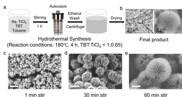
Figure 3. Synthesis of hedgehog particles. a. Schematic illustration of the hydrothermal synthesis process for the hedgehog particles. b. SEM images of the final product showing the individual particle. Stirring time c. 1 min, d. 30 min, and e. 60 min, while keeping the other parameters the same, e.g., the reaction temperature, reaction time and precursor ratio of TBT:TiCl 4 at 180°C, 4 h, and 1:0.65, respectively. Scale bar: 2 μm.
