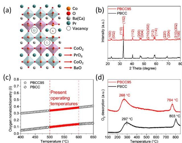
Fig. 1. Material characterization of PBCC and PBCC95 electrodes. (a) schematic of crystal structure for PBCC double perovskite with A-site deficiency; (b) XRD patterns of PBCC and PBCC95; (c) the oxygen non-stoichiometry of PBCC and PBCC95 in temperatures between 400 and 650 °C; (d) O<sub>2</sub>-TPD profiles of PBCC and PBCC95.
