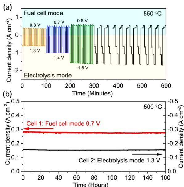
Fig. 5. Reversible operation of the electrochemical cell and long-term stability in fuel cell and electrolysis modes. (a) Reversible operation between electrolysis and fuel cell mode at 550 °C when the cell working voltage is transiently changed; (b) long-term stability testing of the cell in fuel cell mode at 0.7 V and in electrolysis mode at 1.3 V and 500 °C.
