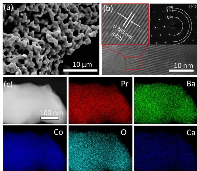
Fig. 2. Morphology and lattice structure of PBCC95 electrode. (a) SEM image of PBCC95 powder; (b) HR-TEM image of PBCC95 particle; (inset) SEAD pattern of PBCC95; (c) EDX-mapping of a PBCC95 particle.
