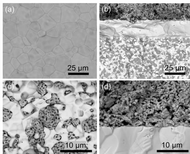
Fig. 6. The morphology of the post-mortem cell. (a) SEM image of electrolyte surface; (b) cross-section image of the interface with PBCC95 oxygen electrode, BCZYb4411 electrolyte, and Ni/BCZYb4411 hydrogen electrode; (c) magnified SEM image in hydrogen electrode with flower-like nickel particles; (d) electrolyte/PBCC95 electrode interface.
