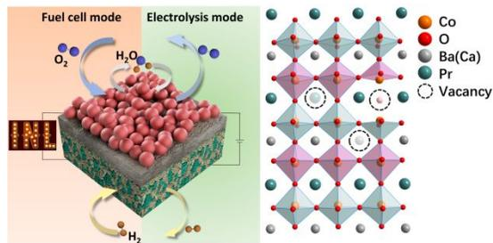
An A-site deficient layered perovskite PBCC95 is developed as a new oxygen electrode incorporated into protonic ceramic electrochemical cell. The cell presents superior electrochemical performances and it can reversibly work between electrolysis and fuel cell mode.
