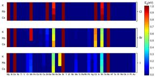
Figure 1: Predicted PBE functional band gaps of the 360 AMX<sub>3</sub> halide perovskite compositions. The top, middle and bottom section correspond to X-site species with halogens X = CI, Br and I, respectively, and in each session, the x and y axes correspond to M and A-site components.
