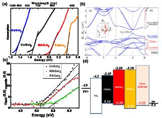
Figure 3. (a) Optical absorption spectrum of CsGel<sub>3</sub>, MAGel<sub>3</sub> and FAGel<sub>3</sub>, in comparison with CsSnl<sub>3</sub>. (b) Calculated band structure and projected density of states of CsGel<sub>3</sub>. The energy of the highest occupied state is set to 0 eV. (c) Photoelectron spectroscopy in air (PESA) of powder samples and (b) Schematic energy level diagram of CsGel<sub>3</sub>, MAGel<sub>3</sub> and FAGel<sub>3</sub>.
