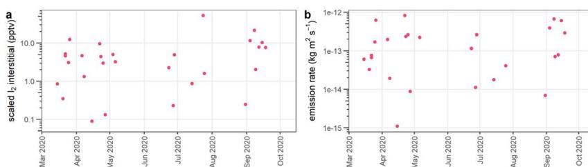
Fig. 7 (a) Interstitial  $I_2$  mixing ratios (in parts per trillion by volume, pptv) predicted from photolysis of iodide, scaled according to interstitial  $I_2$  measurements in Raso (2017).<sup>44</sup> (b)  $I_2$  emission rates, resulting from the calculated interstitial concentrations.
