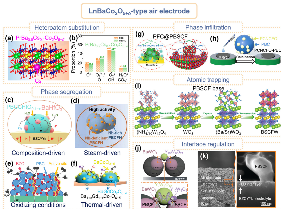
Fig. 10 Recent advances in \text{LnBaCo}_2\text{O}_{5+\delta} -type air electrode materials. (a) Structure of PBCsC, (b) comparisons of different oxygen species contents of PBC and PBCc. Reproduced with permission. 226 Copyright 2023, American Chemical Society. (c) Schematic of Hf-doped \text{PBCCHf}_{0.1} . Reproduced with permission. 229 Copyright 2024, Elsevier. (d) Schematic of PBCFN. Reproduced with permission. 230 Copyright 2022, Wiley-VCH. (e) Schematic of BZO@PBC. Reproduced with permission. 231 Copyright 2022, Wiley-VCH. (f) Schematic of BGCO–BCO hybrid catalyst. Reproduced with permission. 232 Copyright 2024, Wiley-VCH. (g) Schematic of PFC@PBSCF in the presence of contaminants (Cr and steam). Reproduced with permission. 234 Copyright 2022, Wiley-VCH. (h) Schematic for the fabrication procedures of PCNCFO–PBC. Reproduced with permission. 235 Copyright 2024, Wiley-VCH. (i) Structural evolution during reverse atom capture process. Reproduced with permission. 150 Copyright 2024, Wiley-VCH. (j) Mechanism underlying the thermo-mechanical enhancement of TEC gradient formation. Reproduced with permission. 382 Copyright 2024, Wiley-VCH. (k) Cross-sectional SEM image of PBSCF/BZCYyb composite interlayer. Reproduced with permission. 236 Copyright 2024, Wiley-VCH.
