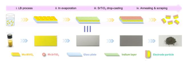
Fig. 11 Schematic illustration for the preparation procedures of Mo:BiVO<sub>4</sub>/In@InOx/Rh:SrTiO<sub>3</sub> electrode particles.<sup>61</sup>
