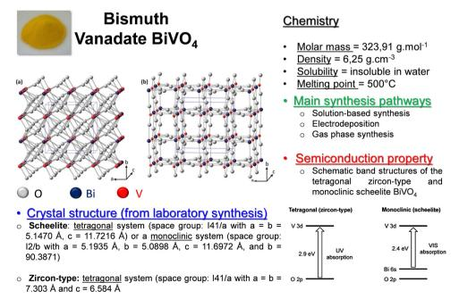
Fig. 7 The identity of the BiVO<sub>4</sub> compound with its main physico-chemical characteristics and properties, crystal structures, and band gap diagram is from Park et al.15
