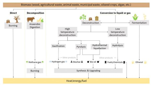
Fig. 2 Global view of transformations of biomass to biofuel processes.<sup>24</sup>
