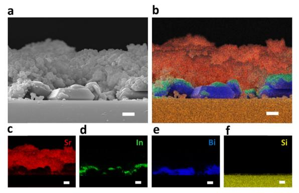
Fig. 12 Cross-sectional SEM (a) and (b)-(f) corresponding EDS mapping images of annealed electrode particle before being scraped from the glass plate. Scale bars, 1 µm.61
