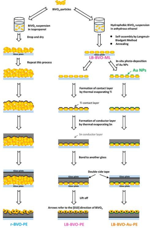
Schematic diagram of the particle transfer (PT) method for preparation of r-BVO-PE, LB-BVO-PE, and LB-BVO-Au-PE.
