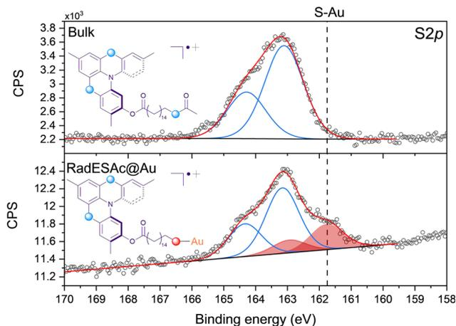
Fig. 1 *S*2*p* XPS region acquired on the **RadESAc** bulk sample (top) and on the **RadESAc@Au** monolayer deposited on Au(111). The dashed line highlights the position of the component attributed to the formation of S–Au bond.
