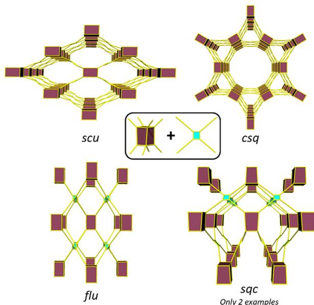
**Fig. 1** Representations of the four different topologies that can be formed from a cubic 8-connected cluster and a tetraptopic linker (with either a tetrahedral or square planar geometry). The maroon polyhedron represents the cluster and the blue shaded rectangle or polygon with yellow lines represents the organic linker.
