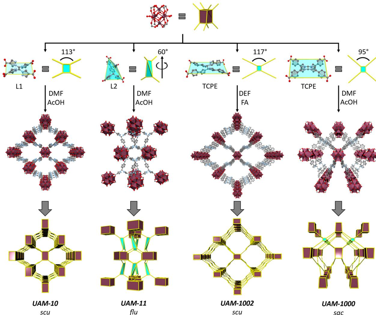
Fig. 3 A summary of the synthesis, structure and topologies of UAM-10, UAM-11, UAM-1002 and UAM-1000. All four MOFs are formed from the same 8-connected cubic Zr-cluster but different linkers and linker conformations lead to the formation of different MOF topologies, in part governed by the restrictions on linker flexibility. The maroon polyhedron represents the cluster and the blue shaded rectangle/polyhedron with yellow lines represents the organic linker.
