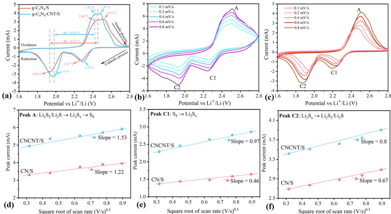
Fig. 5 (a) CV profiles for  $g\text{-C}_3\text{N}_4/\text{S}$  and  $g\text{-C}_3\text{N}_4\text{-CNT}/\text{S}$  cathodes; CV curves at different scan rates for (b)  $g\text{-C}_3\text{N}_4\text{-CNT}/\text{S}$  and (c)  $g\text{-C}_3\text{N}_4/\text{S}$ ; plots of the peak currents versus the square root of scan rates from the CV curves of  $g\text{-C}_3\text{N}_4\text{-CNT}/\text{S}$  and  $g\text{-C}_3\text{N}_4/\text{S}$  cathodes for (d) Peak A, (e) Peak C1 and (f) Peak C2.
