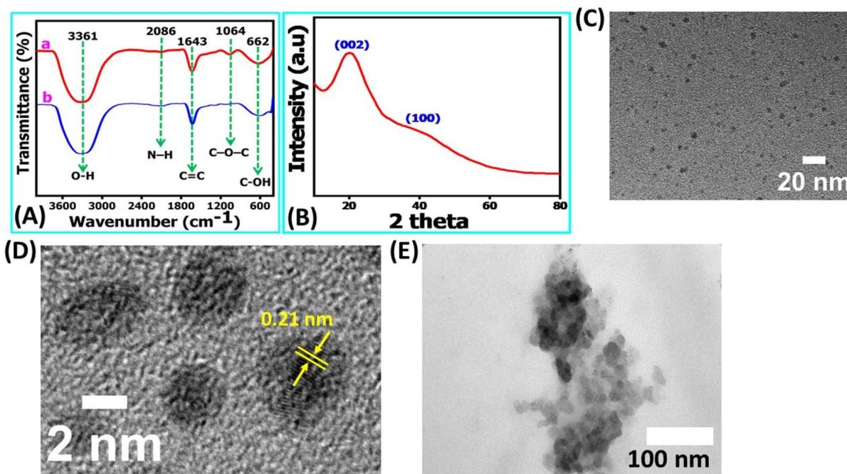
Fig. 2 Characterization and morphological analysis of NR-CDs and their interaction with  $\text{Fe}^{2+}$  ions. (A) FT-IR spectra of neem resin extracts (dark red line) and the NR-CDs (dark blue line). (B) XRD pattern and (C and D) TEM image of the NR-CDs. (E) TEM image of NR-CDs in the presence of  $62 \mu\text{M}$  of  $\text{Fe}^{2+}$  ions.
