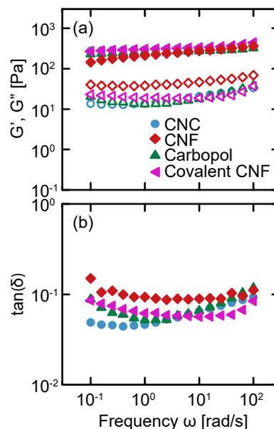
Fig. 2 Storage (closed symbols)  $G'$  and loss (open symbols)  $G''$  moduli and (b)  $\tan(\delta) = G''/G'$  as a function of frequency  $\omega$  for the four classes of gels: CNC, entangled CNF, Carbopol, and covalent CNF.
