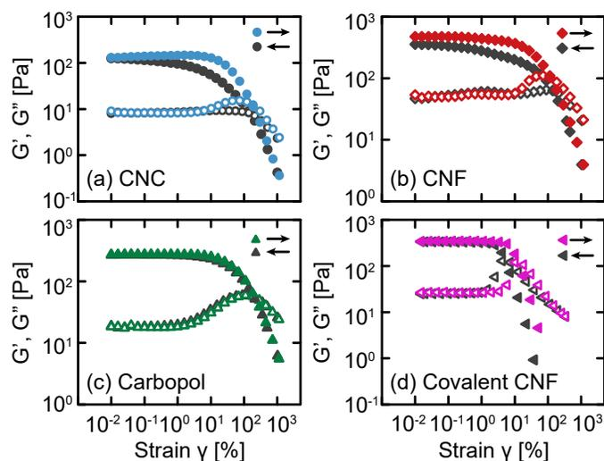
Fig. 3 Storage (closed symbols)  $G'$  and loss (open symbols)  $G''$  moduli as a function of oscillation strain  $\gamma$  for the four classes of gels: (a) CNC, (b) entangled CNF, (c) Carbopol, and (d) covalent CNF. Data collected with increasing and decreasing  $\gamma$  are shown in color and gray, respectively.
