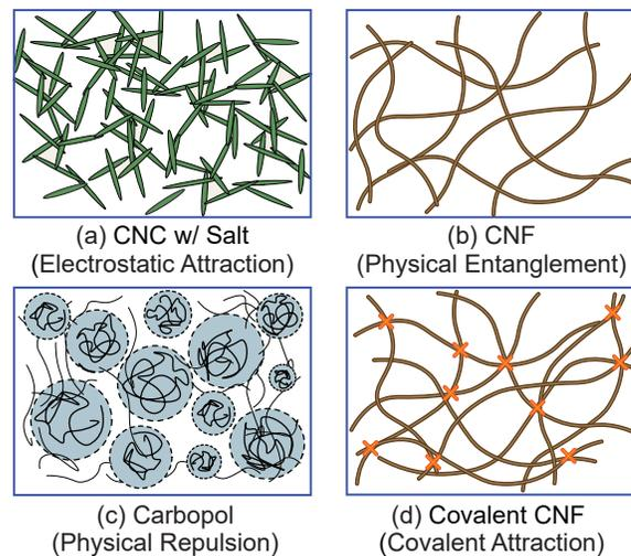
Fig. 1 Schematic illustrating the structures for the four classes of gels: (a) a CNC gel experiencing electrostatic attractions, (b) a CNF gel with physical entanglements, (c) a Carbopol gel with physical repulsion, and (d) a CNF gel with covalent crosslinks.
