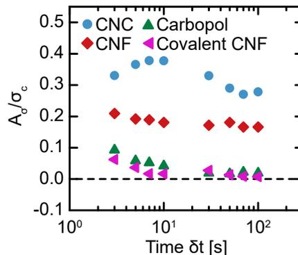
Fig. 9 Normalized hysteric area  $A_\sigma/\sigma_c$  as a function of the time interval per step  $\delta t$  in flow sweeps for different gel classes.
