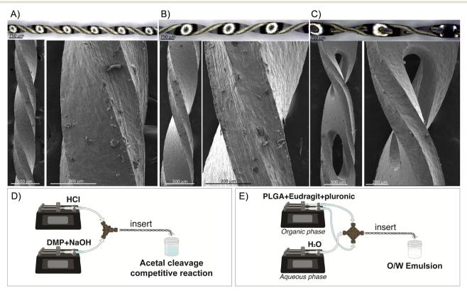
Fig. 1 Representative optical and electronic images of the helical inserts designed in this work to be housed in PTFE tubings with an internal diameter of 0.02" (A), 0.03" (B), and 0.04" (C). D and E present schematics of the setup for the study of the acetal cleavage competitive reaction (D) and the O/W simple emulsification process (E). In both cases, the insert was placed at the outlet tubing.
