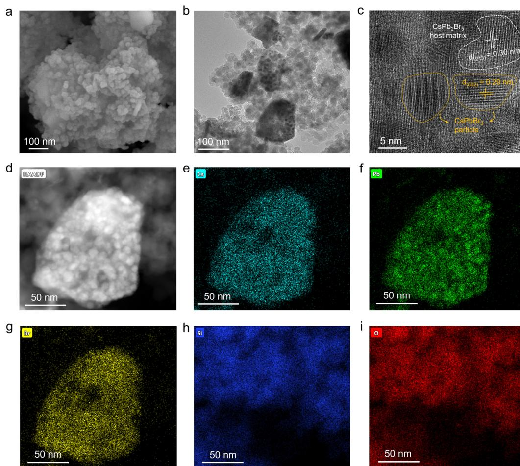
Fig. 2 Microstructural characterization of H-CPB composites. (a) Typical SEM images of H-CPB. (b) SEM images of H-CPB. (c) HRTEM image of  $\text{CsPbBr}_3$  NCs embedded in  $\text{CsPb}_2\text{Br}_5$ . (d)–(i) HAADF-STEM image and the corresponding elemental mapping images showing the elemental distribution of Cs, Pb, Br, Si, and O.
