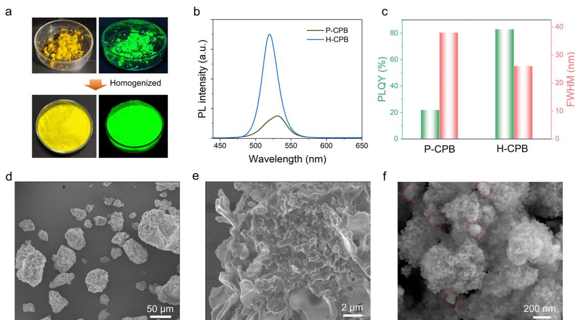
Fig. 3 Improving the homogeneity and PLQYs of CPB composites assisted by SiO<sub>2</sub> nanospheres. (a) Photographs of P-CPB (top) and H-CPB (bottom) under the irradiation of daylight and UV light (right, 365 nm). (b) PL spectra of P-CPB and H-CPB. (c) PLQY value and FWHM of P-CPB and H-CPB. (d) Typical SEM image of P-CPB. (e) High-magnification SEM image of P-CPB. (f) Typical SEM image of H-CPB composites.
