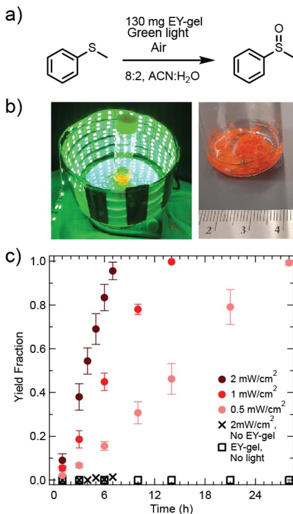
Fig. 2 (a) Reaction schematic for oxidation of thioanisole. (b) Photographs of the light bath reaction setup at  $1 \text{ mW cm}^{-2}$  (left), and the EY-gel in reaction solution (right). (c) Yield fraction as a function of reaction time for the oxidation of thioanisole ( $0.67 \text{ mmol}$ ) using  $130 \text{ mg}$  of EY-gel under varied intensities of green light irradiation ( $\lambda_{\text{max}} = 520 \text{ nm}$ ) at room temperature.
