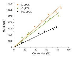
Fig. 2 Number-average molar mass  $(M_n)$  plotted against monomer conversion for the ROP of  $\gamma C_{18}CL$ ,  $\epsilon C_{18}CL$  and  $\beta/\delta C_{18}CL$  isomers using DPP (10 mol%) and 4-methoxybenzyl alcohol as initiator ( $[M]_0/[I]_0 = 50$ ). Number-average molar mass (M<sub>n</sub>) determined by SEC analysis in CHCl<sub>3</sub> (0.5% NEt<sub>3</sub>), calibrated against polystyrene standards.
