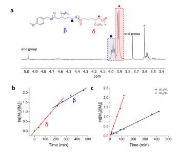
Fig. 3 (a) <sup>1</sup>H NMR spectrum (CDCl<sub>3</sub>, 400 MHz) of  $\beta$  and  $\delta$ C<sub>18</sub>PCL. \* = MeOH. (b) Semi-logarithmic kinetic plot time for the ROP of  $\beta/\delta C_{18}CL$ isomers. (c) Resolved semi-logarithmic kinetic plot for the ROP of  $\beta$ /  $\delta C_{18}CL$  isomers. [M]<sub>0</sub> = 0.5 M (calculated by NMR spectroscopy based on a starting ratio of  $\beta$  isomer :  $\delta$  isomer = 1 : 1).
