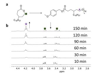
Fig. 1 (a) ROP of  $\gamma C_{18}CL$  using DPP (10 mol%), 4-methoxybenzyl alcohol ([M] $_0/[I]_0$  = 50), benzene- $d_6$ . (b) Stacked  $^1H$  NMR spectra (benzene- $d_6$ , 300 MHz) during ROP of  $\gamma C_{18}CL$  showing the  $CH_2OC = O$  monomer resonance between  $\delta$  = 3.37–3.70 ppm and  $CH_2OC = O$  polymer resonance at  $\delta$  = 4.2 ppm.
