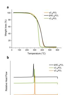
**Fig. 5** (a) Thermogravimetric analysis (TGA) of  $\gamma C_{18}$ PCL,  $\epsilon C_{18}$ PCL and  $\beta / \delta C_{18}$ PCL isomers. Analytical data of the analysed polymers is summarised in Table 1. (b) Differential scanning calorimetry (DSC) for 2<sup>nd</sup> cooling cycle (200 to -100 °C, 10 °C min<sup>-1</sup>) showing crystallisation and melting temperature of the polymers.
