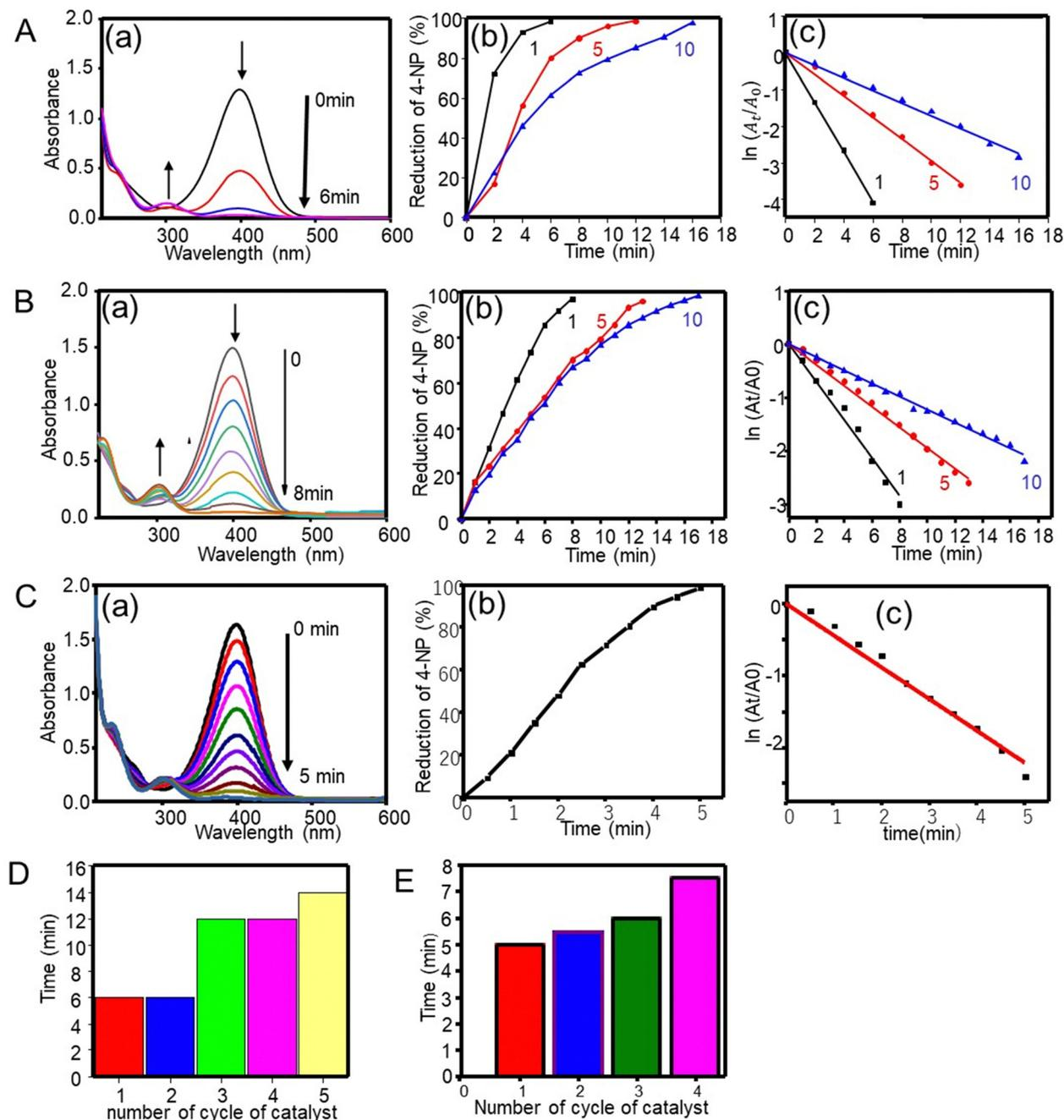
**Fig. 3** (A) (a) UV-visible absorption spectra of the hydrogenation reaction of 4-nitrophenol by NaBH<sub>4</sub> using a silver catalyst (1-min irradiation): (b) percentage of reduction and (c)  $\ln(A_t/A_0)$  versus reaction time using different silver catalysts (1, 5 and 10 min irradiation). Corresponding spectra and plots obtained using (B) gold catalysts and (C) the Ag@CNF filament. Recyclability of (D) the silver catalyst (1 min irradiation) and (E) the Ag@CNF filament.
