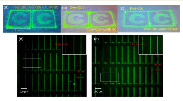
Fig. 5 The photographic images of the patterned PQD-PNC films under irradiation from a UV lamp. (a-c) The PQD-PNC films comprising (a) Oct-QDs and AuNP-GO; (b) OAm-QDs and AuNP-GO; (c) Post-QDs and AuNP-PEGGO. The substrate size was  $3 \times 3$  cm for all samples. Microscale patterns of the PeQD-PNC films prepared with (d) Post-QDs; (e) Post-QDs and AuNP-PEGGO. The insets show the magnified view of the line patterns, enlarged from the white squares in (d) and (e), respectively.
