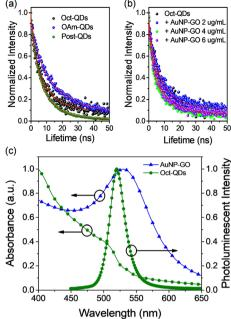
Fig. 3 Photoluminescence decay of the FAPbBr<sub>3</sub> quantum dots in toluene solutions. (a) The decay curves of Oct-QDs, OAm-QDs and Post-QDs; (b) the decay profiles of the Oct-QDs mixed with varying concentrations of AuNP-GO NPs. All the samples were excited with a 375 nm pulsed laser. (c) Photoluminescence spectrum of Oct-QDs and plasmonic absorption of AuNP-GO.
