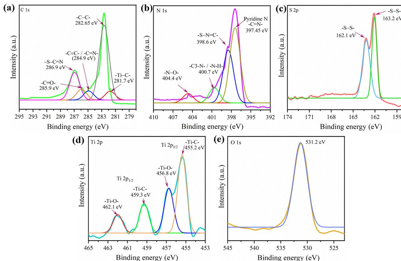
Fig. 2 (a–e) XPS spectrum showing the complete scan and the corresponding spectra for the elements present in the  $g\text{-C}_3\text{N}_4\text{-Mx/S}$  composite.
