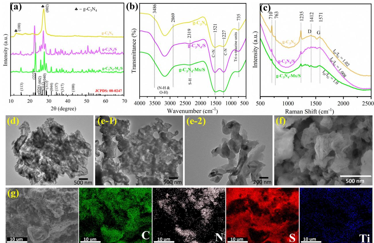
Fig. 1 (a) XRD patterns, (b) FTIR spectra, and (c) Raman spectra of  $g\text{-C}_3\text{N}_4$ ,  $g\text{-C}_3\text{N}_4/\text{S}$ , and  $g\text{-C}_3\text{N}_4\text{-Mx/S}$ . TEM images of (d)  $g\text{-C}_3\text{N}_4$  and (e)  $g\text{-C}_3\text{N}_4\text{-Mx/S}$  materials. (f) SEM images of  $g\text{-C}_3\text{N}_4\text{-Mx/S}$ . (g) Color mapping of  $g\text{-C}_3\text{N}_4\text{-Mx/S}$  demonstrating the uniform distribution of C, N, S, and Ti elements.
