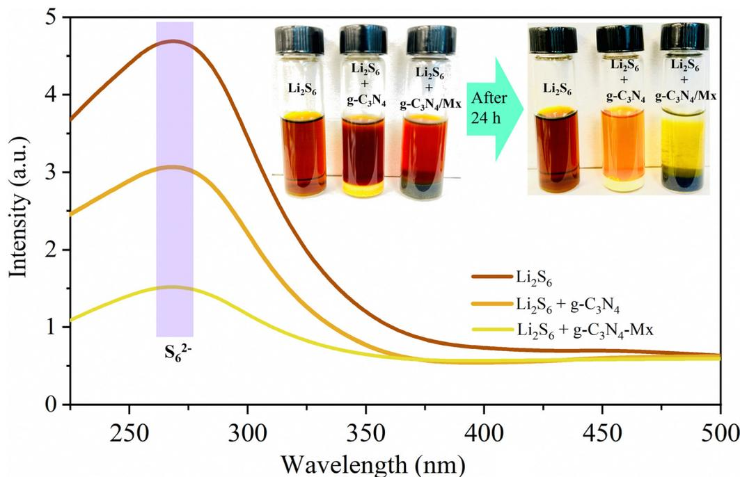
Fig. 3 UV-Vis spectra for blank  $\text{Li}_2\text{S}_6$  and  $\text{Li}_2\text{S}_6$  added with  $\text{g-C}_3\text{N}_4$  and  $\text{g-C}_3\text{N}_4\text{-Mx}$  (after 24 h). The inset shows the digital picture of the effect of active materials on the adsorption of LiPSs in  $\text{Li}_2\text{S}_6$  solution.
