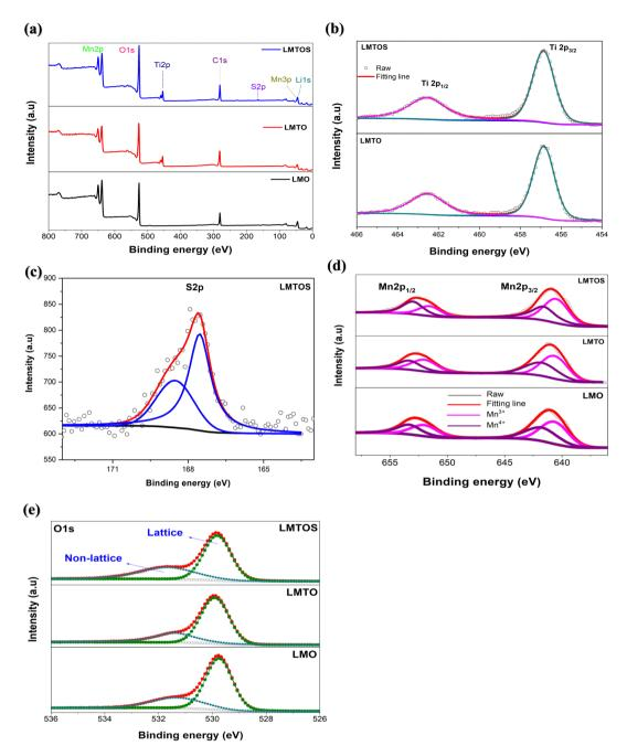
Fig. 6 XPS spectra for particles: (a) full spectra, (b) Ti 2p, (c) S 2p, (d) deconvoluted profiles of Mn  $2p_{3/2}$  and (e) the O 1s XPS spectrum.
