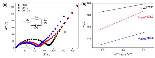
Fig. 9 EIS of the cathodes after 10 cycles of GCC test at 10C over a frequency range of 0.1-1 MHz at the OCP (V) state; (b) corresponding linear fitting curve of Z' vs.  $\omega^{-1/2}$  at low frequencies.
