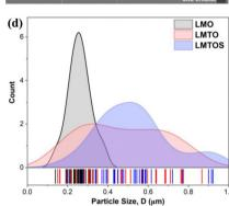
Fig. 3 FE-SEM surface images of (a) LMO, (b) LMTO, (c) LMTOS particles (scale bar in all images: 2 µm), and (d) particle-size distribution for three synthesized particles. LMO, LMTO, and LMTOS are depicted by the black, red, and blue curves, respectively.
