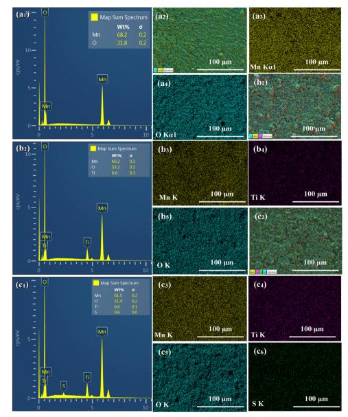
Fig. 2 FE-SEM with EDS results of (a1) LMO, (b1) LMTO, and (c1) LMTOS particles. EDS mapping results: (a1) LMO, (b1) LMTO, and (c1) LMTOS (Mn ((a2), (b2), and (c2)); Ti ((b3) and (c3)); O ((a3), (b4); and (c4)); and S (c5)).
