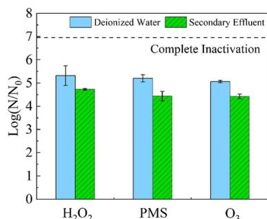
Fig. 3 Inactivation efficiency of MS2 coliphage using O<sub>3</sub> (0.1 mM), PMS (1 mM), and H<sub>2</sub>O<sub>2</sub> (50 mM) with a contact time of 30 min in DI water and secondary effluent.
