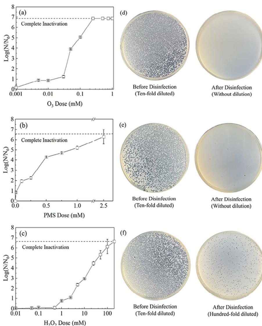
Fig. 1 Inactivation efficiency of MS2 coliphage in 30 min with different oxidants (a) O<sub>3</sub> (0.001–1 mM), (b) PMS (0.01–2.5 mM), (c) H<sub>2</sub>O<sub>2</sub> (0.01–200 mM); (d–f) culture plates of MS2 coliphage treated with 1 mM (d) O<sub>3</sub>, (e) PMS, and (f) H<sub>2</sub>O<sub>2</sub>.
