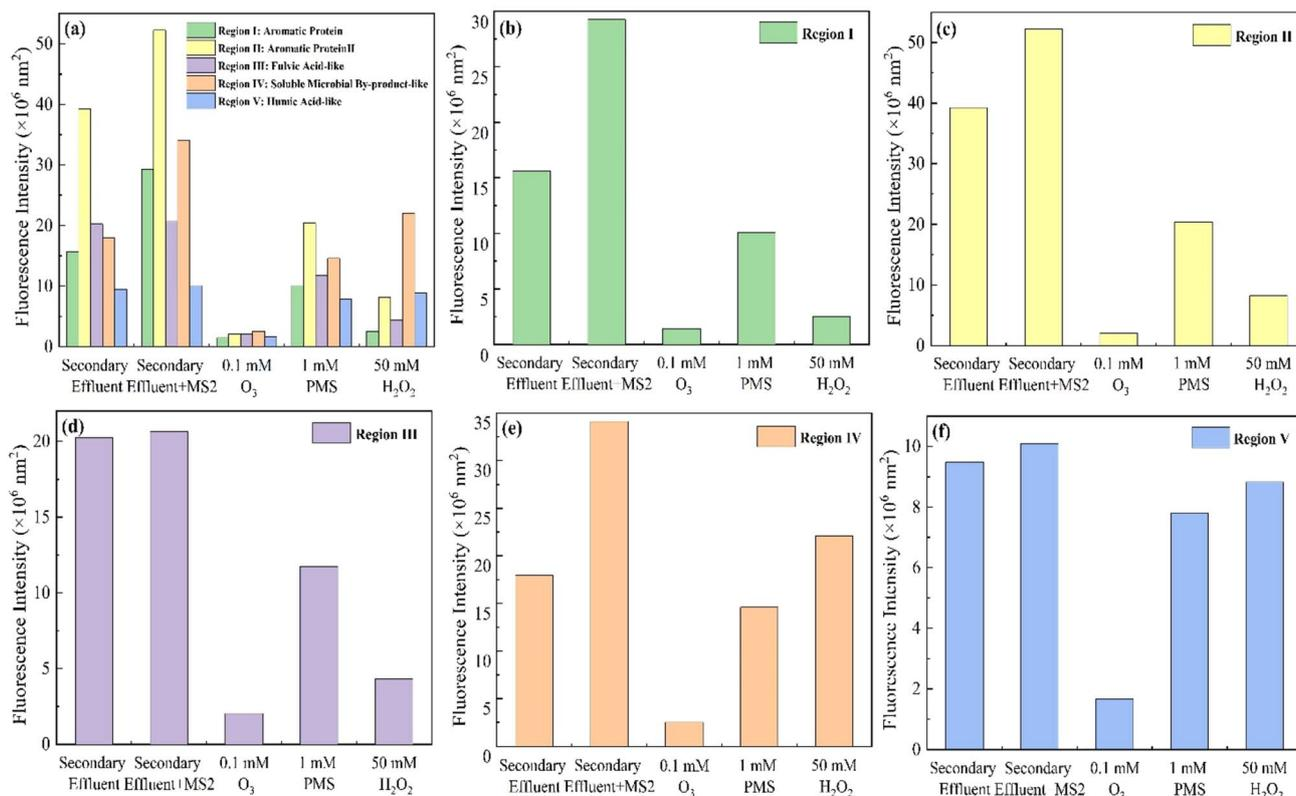
Fig. 5 Fluorescence intensity of secondary effluent, secondary effluent with MS2 coliphage, and secondary effluent with MS2 coliphage after disinfection within 30 min with 0.1 mM  $O_3$ , 1 mM PMS, and 50 mM  $H_2O_2$ . (a) 5 FRI regions; (b) region I; (c) region II; (d) region III; (e) region IV; (f) region V.
