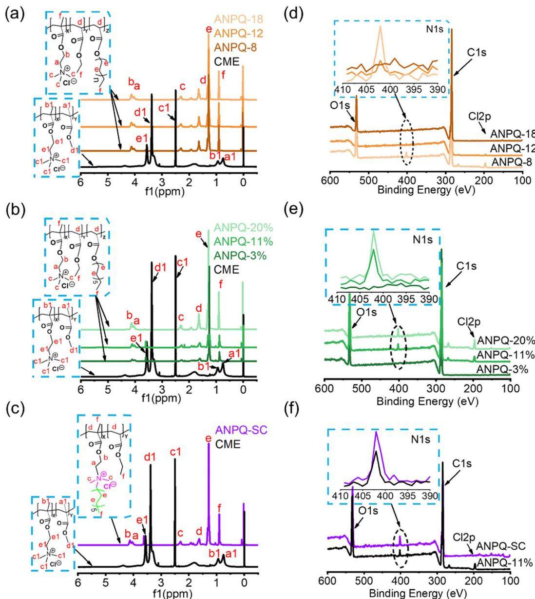
Fig. 1 Synthesis and characterization of ANPQ. (a–c) <sup>1</sup>H NMR of ANPQs. (d–f) XPS of ANPQs.
