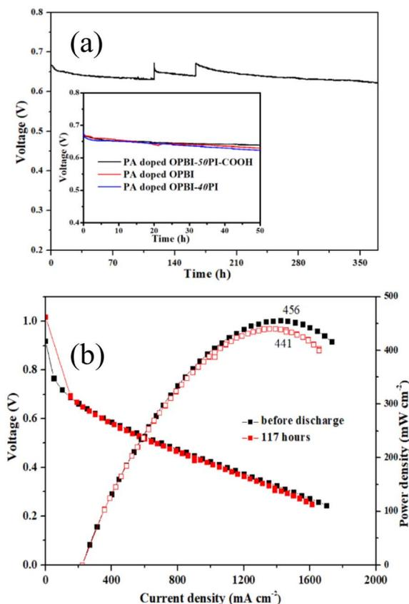
Fig. 9 (a) Short-time durability test of a PA-doped membrane fuel cell with an identical current density of 150 mA cm<sup>-2</sup> operated without humidity and backpressure at 140 °C; (b) polarization and power density curves at different operating times for cells with a PA-doped OPBI-50PI-COOH membrane at 140 °C with gas flows of 80- and 160 mL min<sup>-1</sup> for dry H<sub>2</sub> and O<sub>2</sub> without backpressure.
