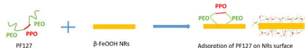
Fig. 6 Schematic illustration of the adsorption of the PEO-PPO-PEO block of PF127 on the \beta -FeOOH NR surface.
