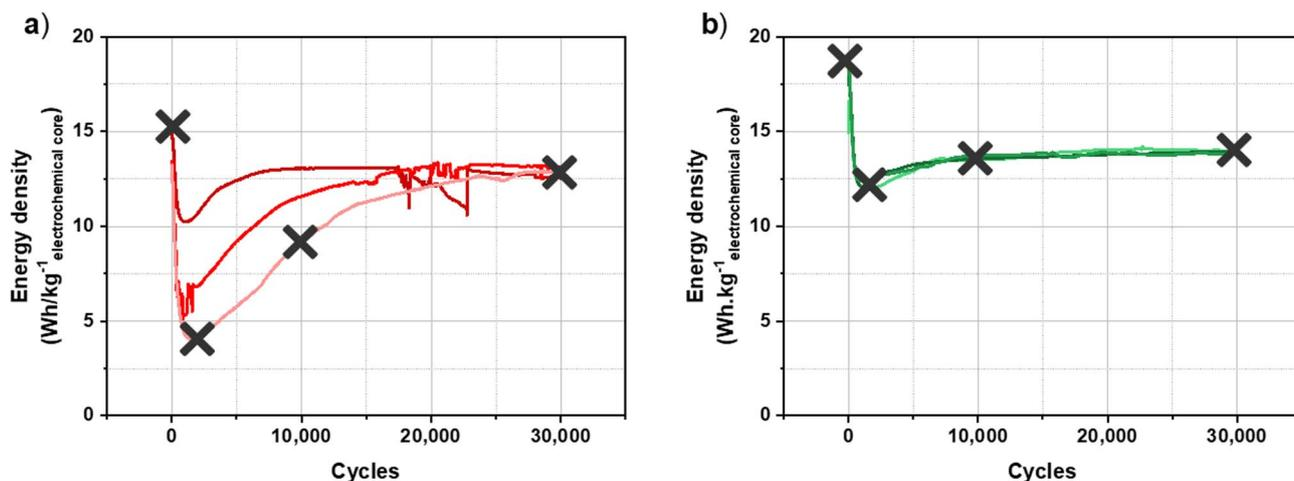
Fig. 5 Long-term cycling of a hybrid KIC in 0.8 mol L<sup>-1</sup> KPF<sub>6</sub> AN at 16 mA cm<sup>-2</sup> between 0.5 and 3.5 V at room temperature in the pouch cell configuration after CC formation (a) and after CV formation (b).<sup>8</sup>
