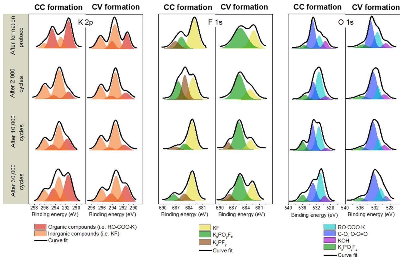
Fig. 6 High-resolution K 2p, F 1s and O 1s XPS spectra obtained on the graphite electrode surface after CC formation and CV formation, after 2000, 10 000 and 30 000 cycles at  $16 \text{ mA cm}^{-2}$  at room temperature.
