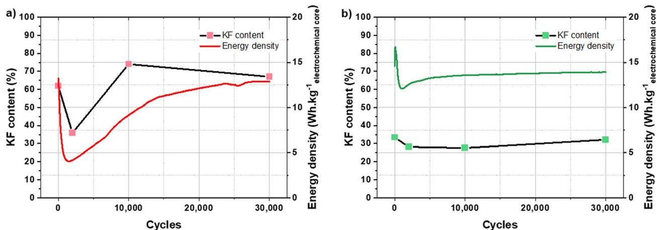
Fig. 8 Evolution of KF content in the SEI and energy density of a KIC cell during cycling at 16 mA cm<sup>-2</sup> at room temperature after CC formation (a) and after CV formation (b).
