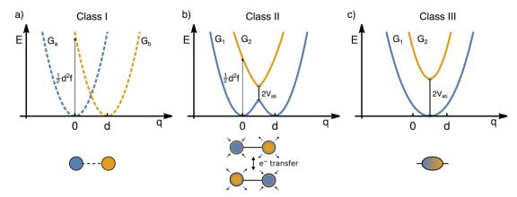
Fig. 1 One dimensional potential curves of Robin–Day classes ((a) class I, (b) class II, (c) class III) separated along the ET coordinate (q). The vertical arrow of length  $\frac{1}{2}d^2f$  represents the reorganization energy.  $V_{ab}$  is the potential coupling between the initial diabatic states  $G_a$  and  $G_b$  that leads to the adiabatic states  $G_1$  and  $G_2$ .
