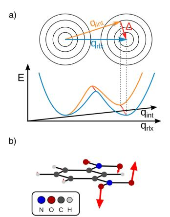
Fig. 7 (a) Schematic representation of the separable intrinsic ET coordinate (Marcus dimension,  $q_{\rm int}$ , orange) and orthogonal structural relaxation ( $\Delta$ , red arrow) vs. the relaxed ET coordinate ( $q_{\rm rlx}$ , blue) that may be obtained from a LICC approach. (b) Structural relaxation obtained by LICC between the second minimum at the Marcus dimension and fully optimized geometry.
